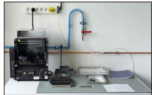
Gross leaks tests station
