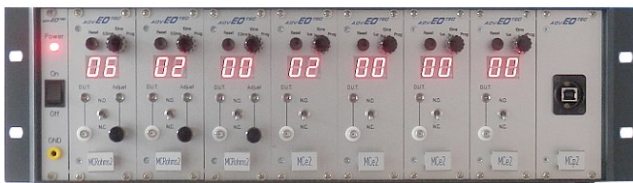
MCROhms2/MCE2 electrical modules configuration And MCP2 communication module Rack for bay
